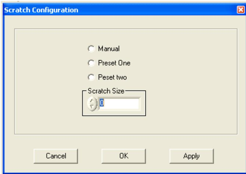
This screen capture is of the user interface to set the maximum allowable scratch size.
