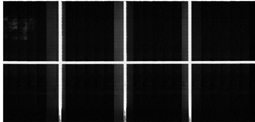
The camera (s) capture samples shown in (Fig 1) as the panel travels past the camera view, The samples are indexed by the encoder and reconstructed by the Computer to create the test image.
